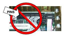
If installed wrong, the connector will be to one side and pins will be exposed.
