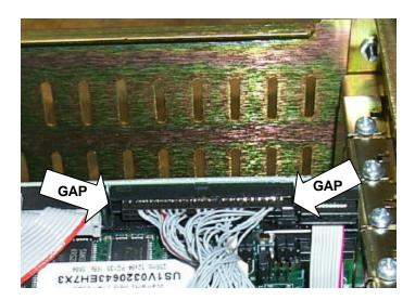
If installed correctly, there will be gaps on either side of the connector.
